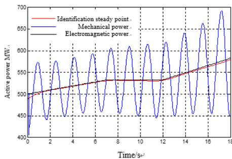
Fig. 2. Comparison chart of the actual steady point and the identified steady point.
