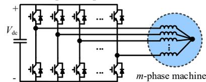
Fig. 11. The topology of one-sided multiphase converters with one neutral point.
