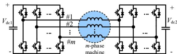
Fig. 10. The topology of open-winding multiphase converters with two DC voltage sources.
