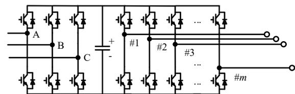
Fig. 6. The topology of AC-DC-AC multiphase converters.
