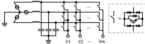
Fig. 7. The topology of direct matrix multiphase converters.
