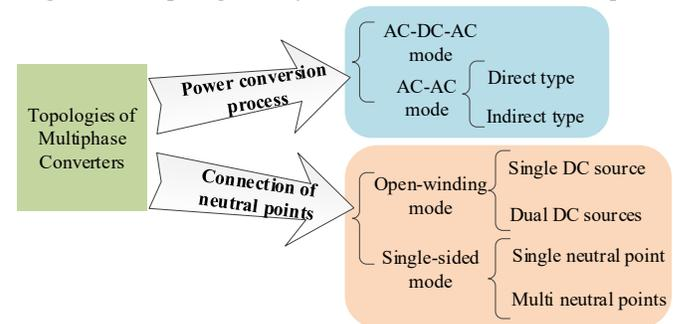
Fig. 5. Classification of multiphase converter topologies.
