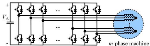
Fig. 12. The topology of one-sided multiphase converters with multiple neutral points.
