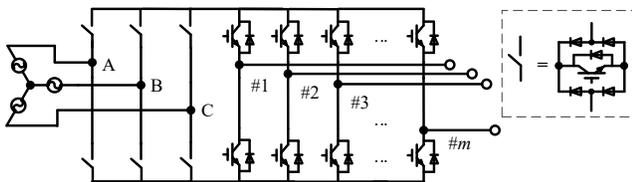
Fig. 8. The topology of indirect matrix multiphase converters.
