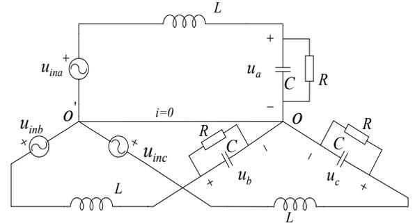
Fig. 4. Three-phase extended equivalent circuit.
