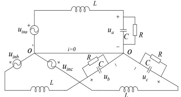
Fig. 4. Three-phase extended equivalent circuit.
