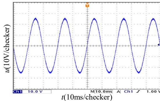
Fig. 20. The output voltage waveform for rectifier load.
