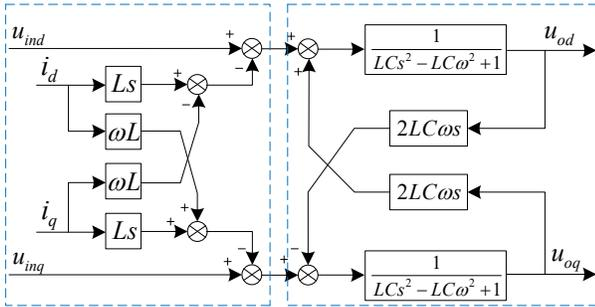
Fig. 9. The mathematical model of the single-phase inverter.
