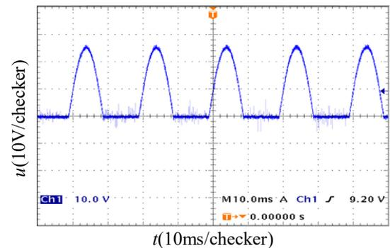
Fig. 21. The voltage waveform across the resistor of the rectifier load.
