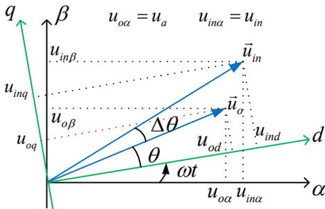
Fig. 6. The vector diagram of  $dq$  coordinate system.
