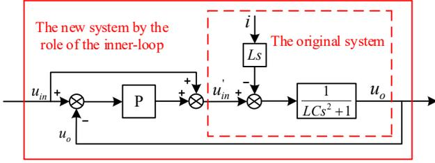
Fig. 12. The block diagram of the inner-loop control
