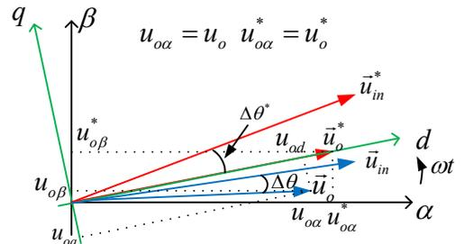
Fig. 8. The vector diagram of the closed-loop control.
