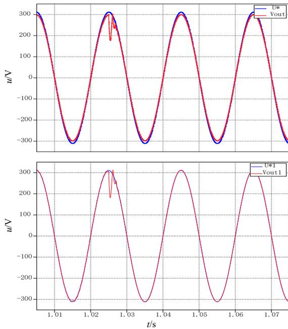
Fig. 15. Simulation waveform comparison of voltage and current dual closed-loop (Top) and voltage dual closed-loop (Lower).
