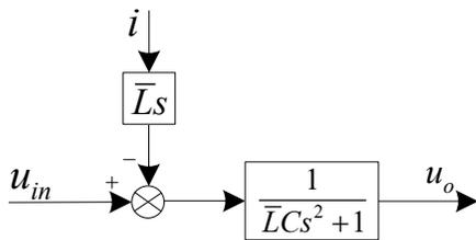
Fig. 13. The equivalent structure of the new system after adding the inner-loop.
