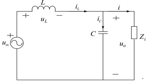
Fig. 2. The equivalent circuit of the single-phase inverter.
