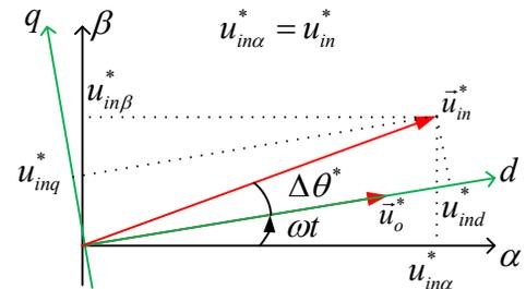
Fig. 7. The vector diagram of the open-loop control.
