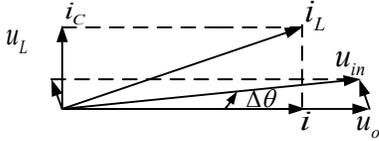
Fig. 3. Phasor diagram of equivalent circuit.
