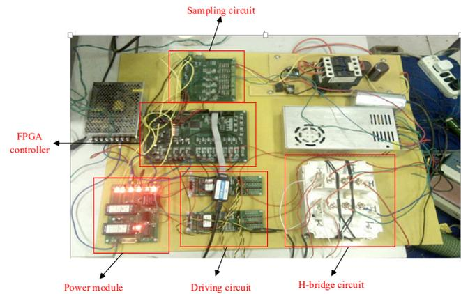
Fig. 17. Experiment platform.
