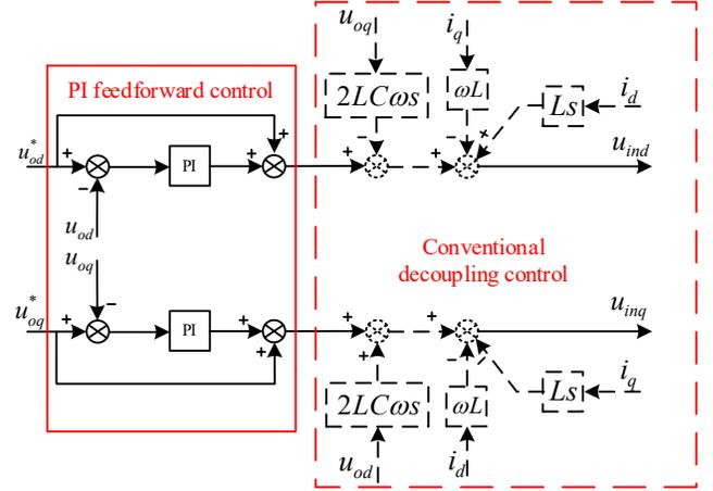
Fig. 10. The block diagram of the outer-loop control.
