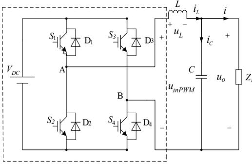
Fig. 1. The circuit diagram of the signal-phase inverter
