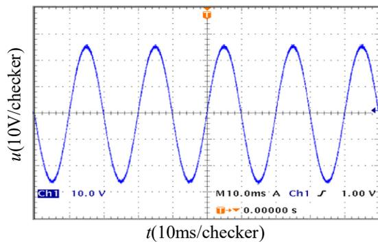
Fig. 19. Full-load inverter output voltage waveform.
