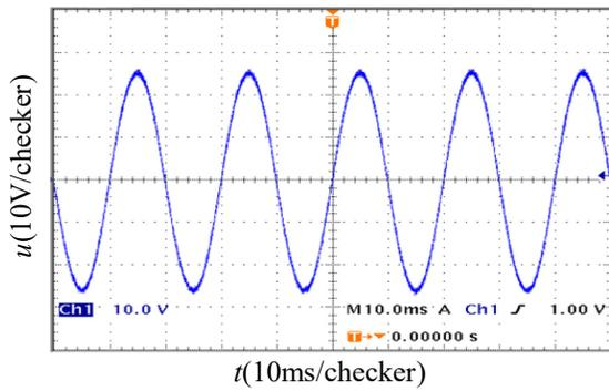
Fig. 19. Full-load inverter output voltage waveform.
