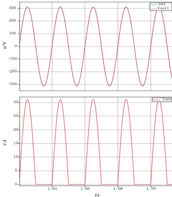
Fig. 16. The output voltage and current waveform with the diode load.
