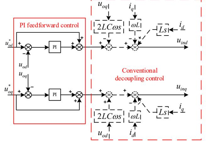
Fig. 10. The block diagram of the outer-loop control.
