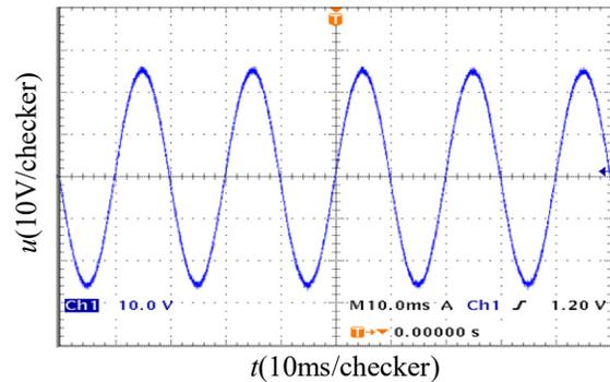
Fig. 18. No-load inverter output voltage waveform.
