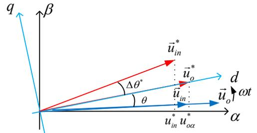
Fig. 11. The vector diagram of the inner-loop control after the load is disconnected
