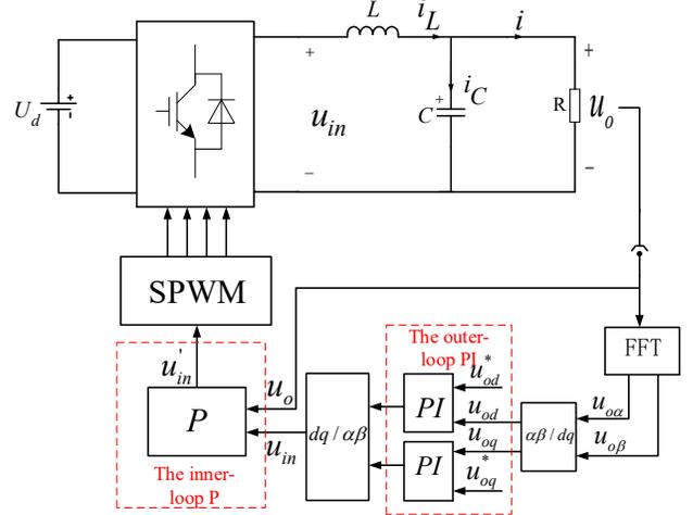
Fig. 14. The system control block diagram.
