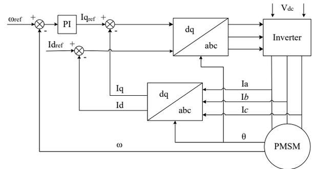
Fig. 7. FOC scheme for the PM TFM.
