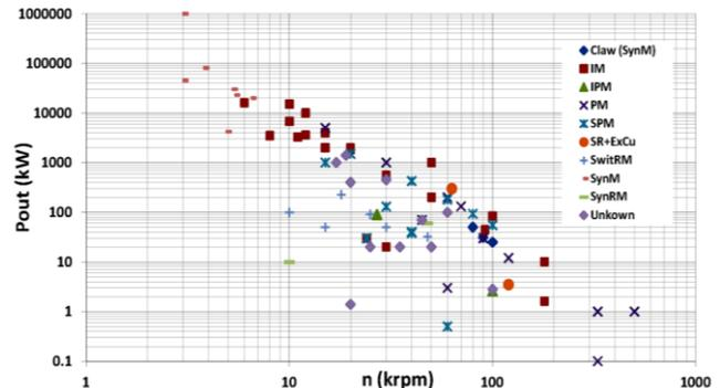
Fig. 2. Survey of high-speed machines by topology [1].
