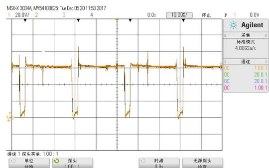
Fig. 19. DC link voltage waveform.
