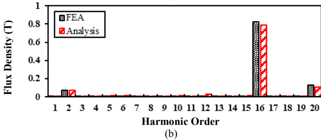
Fig. 5. Air-gap flux density of ST-PMVMs with pole ratio of 16/2.
